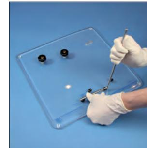
Hold the screw in position and reattach the black turn knob.
