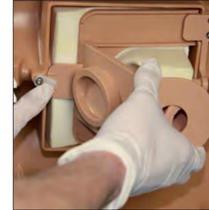
Depress and turn the white retaining clip to release the Frame.
